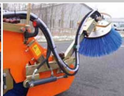
Hydraulic side brush w/hydraulic lifting and lowering
