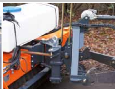
3D hitch system with roller floating tunnel
